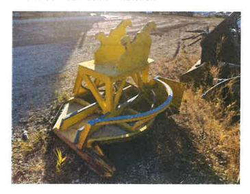
This will cut branches of trees overhanging onto the right of ways but doesn't truly mulch but breaks debris up into chunks. Debris will end up on the road and would have to be cleaned off. Road would have to be blocked off while working due to flying debris. Only one contractor in the Peace country that has one. Cost would be \$12,000.00/km of road plus cleanup of debris and mob and demob. This is just a trimming of overhanging branches which will certainly grow back.
