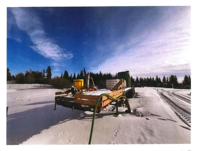
The photos above are of my current tender high boy trailer to the sprayer. I used to have the filter pot at the dugout but then I needed to tender to the field and had some algae in the tanks that was hard to clean out so I just mounted everything on the trailer so I could preclean the water as it was getting loaded to the sprayer.
